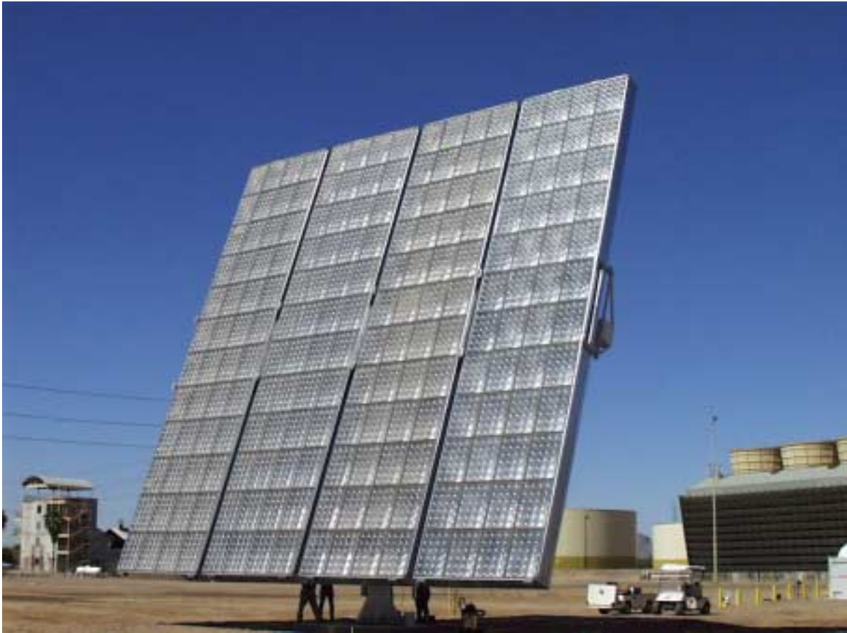
Figure 1: A four MegaModule™ System produces 20,000 watts
